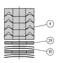
Figure 3. V-Ring Packing Kit
